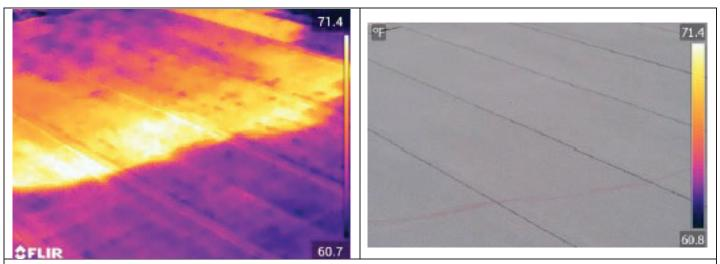
Large puddle like pattern where roof membrane looks unchanging on the surface. Roof structure feels soft in places under membrane.
