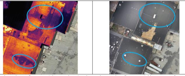
Leaks under roofing material, upper location due to damaged roofing material but extent of water damage would not be known from aerial photo without IR.
