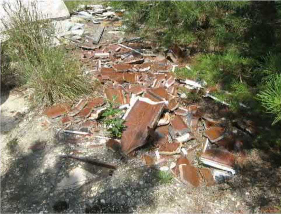
Photograph 11: Debris pile containing demolition debris which may be asbestos containing siding.
